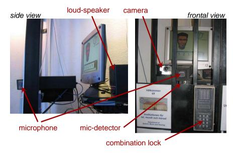
Figure 5.1: The on-site version of PER from side and frontal views. Photos by Botond Pakucs.
