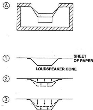
Figure 1.1. Cross-section of a loudspeaker box seen from the side, and stages 1 to 3 described in the text. The arrows mark the position of the loudspeaker membrane in relation to its equilibrium and the varying air pressure (the sound pressure) acting on the paper sheet, respectively.
