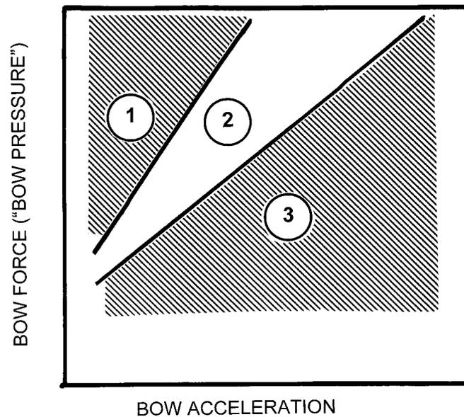
**Figure 8.7.** Typical allowed working range for perfect tone attack (range 2). Range 1 results in non-perfect "prolonged" attacks and range 3 in non-perfect "multiple slip" attacks (after Guettler 2002).
