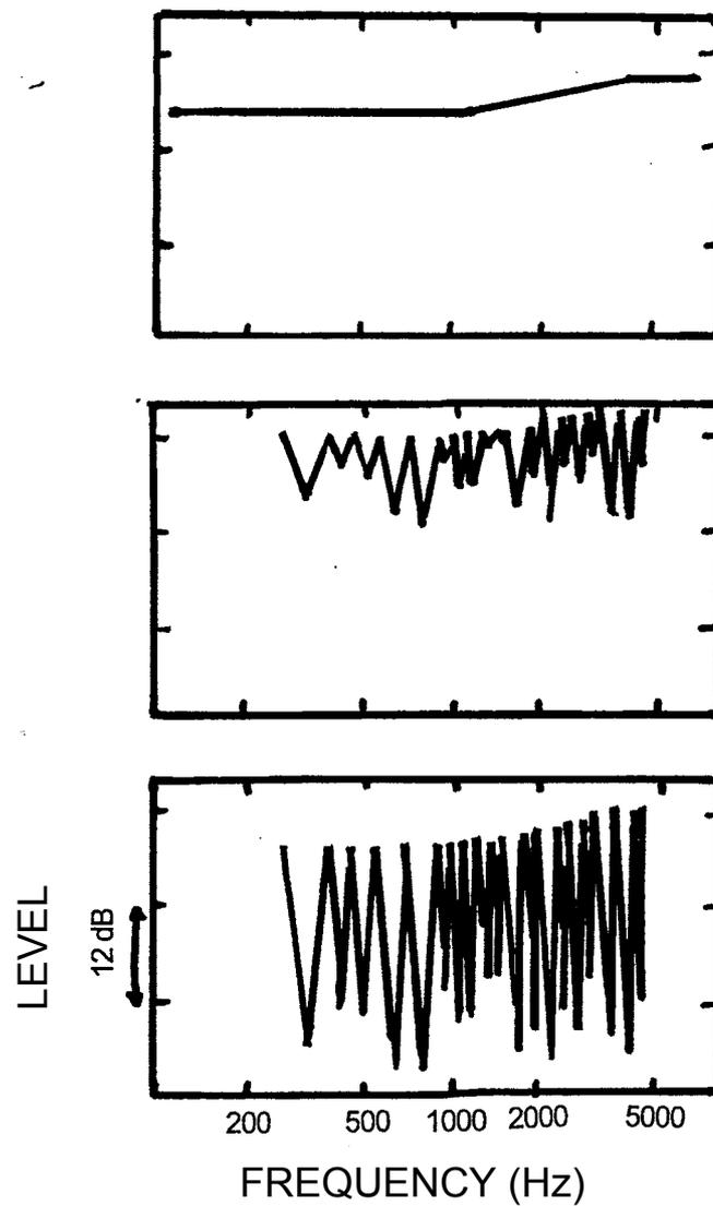
**Figure 8.13.** Different peakiness used in timbre experiments (from Mathews and Kohut).
