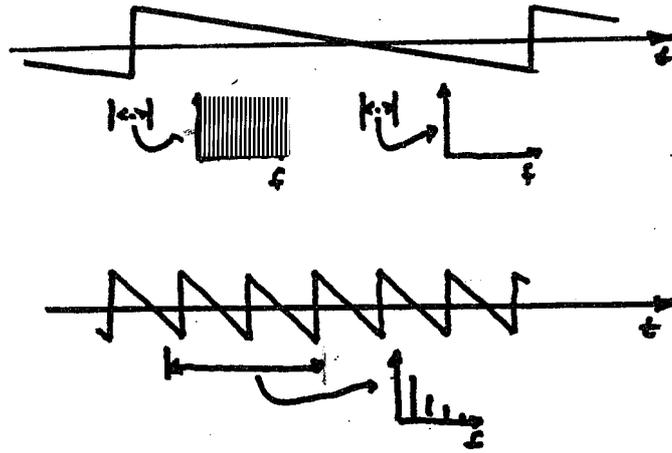
**Figure 8.3.** (Upper part) At very low frequencies a step of the force is caused at every slip and thereafter slowly varying amplitude. A short time window gives a flat pulse spectrum at the step, no spectrum signal between steps, and (lower part) with a time window long compared to the period of the force signal, the normal case, a tone spectrum is obtained.
