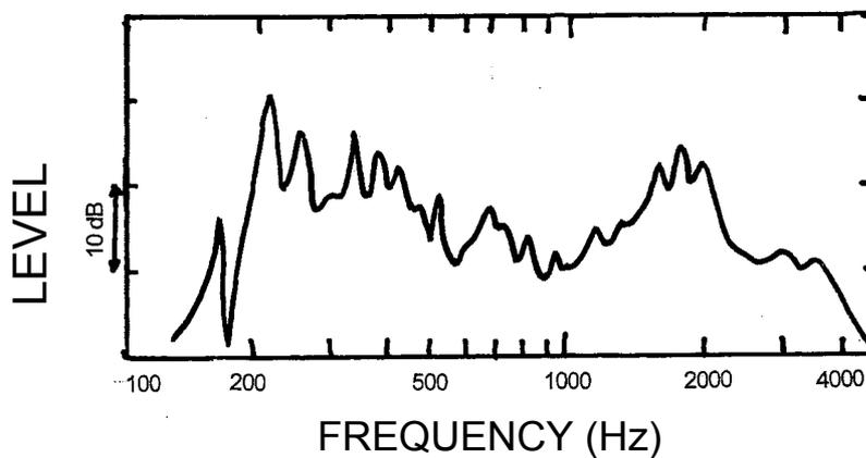
**Figure 8.14.** Vibration sensitivity (mobility) curve for an electronic viola (from Gorrill).
