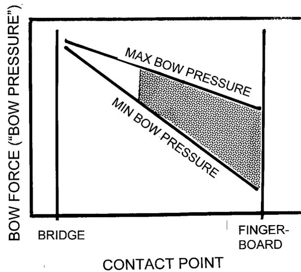
**Figure 8.5.** Allowed working range (shaded area) for "bow pressure" (the force pressing the bow against the string) at different bow contact points (after Schelleng 1973).
