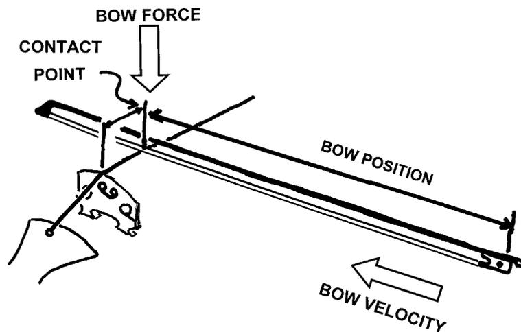
**Figure 8.4.** A violin string is played with a bow. The player controls bow velocity, bow position, bow distance to the bridge (contact point), and the force pressing the bow against the string (the "bow pressure").
