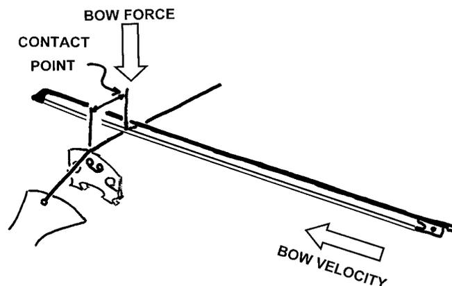
**Figure 8.1.** Physical bowing parameters, bow force (bow pressure), contact point and bow velocity.
