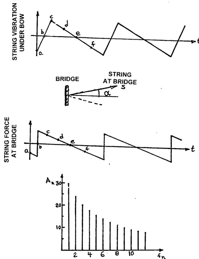
**Figure 8.2.** String motion at contact point, angle variations of string at bridge and string forces at the bridge (all three seen from above), and tone spectrum of bridge force.
