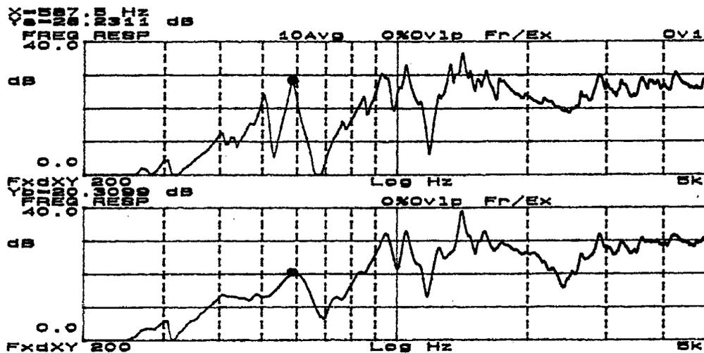
**Figure 8.9.** Vibration sensitivity of a violin free on supports and held for playing – violin Leon Bernardel 1909 with cursor on P2.
