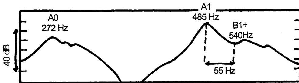
**Figure 8.12.** Examples of vibration sensitivity curves with the new test method: The frequency separation between peak A1 (at 485 Hz) and valley B1 (at 540 Hz) have been marked with a triangle and the separation measured in Hz (after Hutchins).
