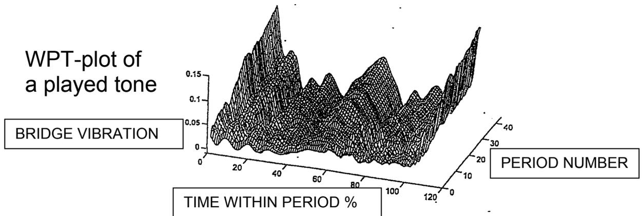
**Figure 8.24.** Time history of a violin tone (bridge vibrations, WPT-plot invented and developed by F. Le Coustumer).
