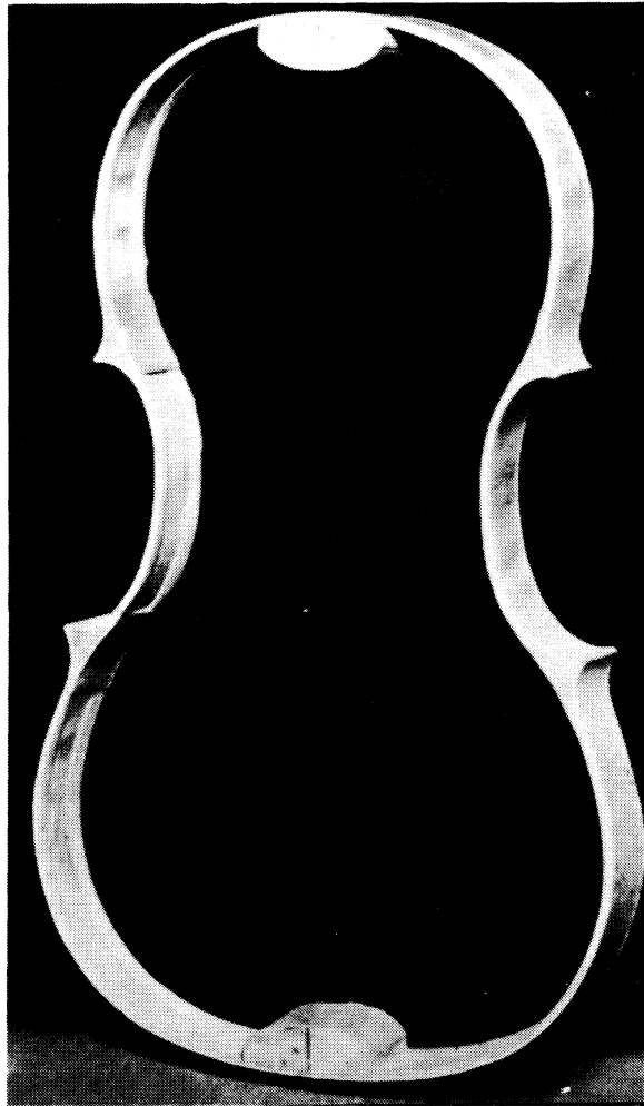
Fig. 7. Finished ribs with cleaned up blocks and linings (from Möckel & Winckel, 1967).
