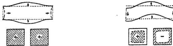
Fig. 1. Two lowest vibrational modes of a box with identical top and bottom plates and perforated sides. (a) Top and bottom move in anti-phase; (b) Main part of top and bottom move in phase but opposite to sides. The in-phase mode will have the higher frequency.
