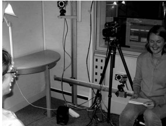
Figure 1 Data collection setup in corpus 1 with video and IR-cameras, microphone and a screen for prompts.
