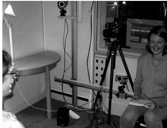
Figure 1 Data collection setup in corpus 1 with video and IR-cameras, microphone and a screen for prompts.
