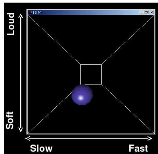
Figure 2 The ExpressiBall: graphical interface for real-time feedback of expressive music performance. Dimensions used in the interface are; X = tempo, Y = sound pressure level, Z = spectrum (attack time & centroid), Shape = articulation, Color = emotion. Left figure shows the feedback for a sad performance. Right figure shows the feedback for an angry performance.
