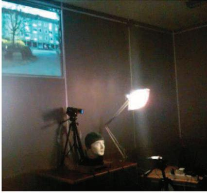
Figure 3: A snapshot of the experimental setup showing a video playing on the wall, and an animated agent being projected on the static head model (3D condition).
