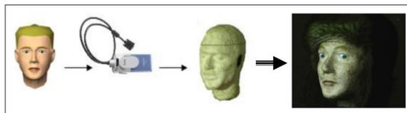
Figure 1: The animated head on the left, projected using the Pico laser projector in the middle, on a static physical head model. The resulted projected face is shown on the right.
