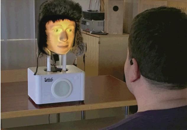
**Fig. 1.** Illustration of the experiment setting with the robot Furhat and a user interacting
