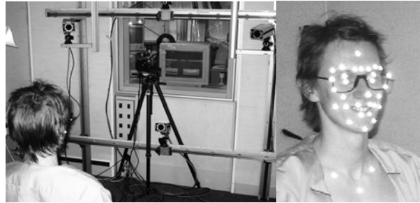
Figure 2. Data collection setup with video, microphone and four IR-cameras and a screen for prompts (left). Facial markers used for the recording (right).
