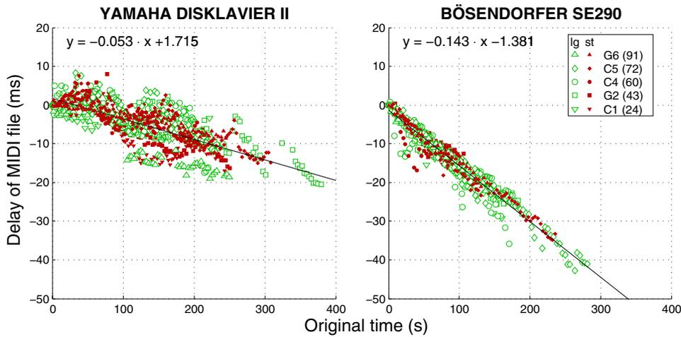
Figure 1: Timing delays (ms) as a function of recorded time (s) between the original recording and the MIDI file as recorded by the computer-controlled grand pianos for two types of touch: *legato* ('lg') and *staccato* ('st'). Negative values indicate that an onset in the MIDI file was earlier than in the original recording. The straight lines are linear fits of the whole data.
