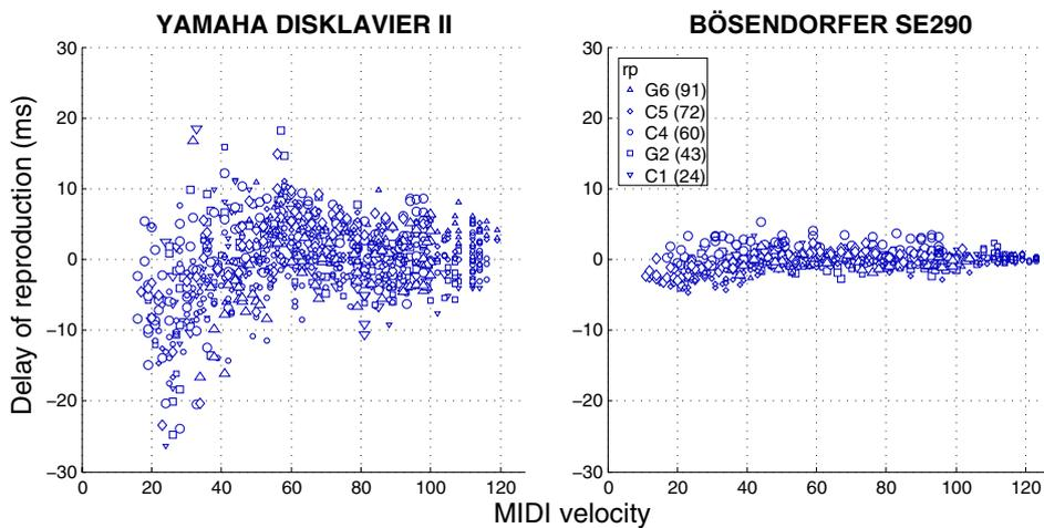
Figure 3: Timing delays (ms) between the original and its reproduction by the computer-controlled piano. (No systematic trend had to be removed.)
