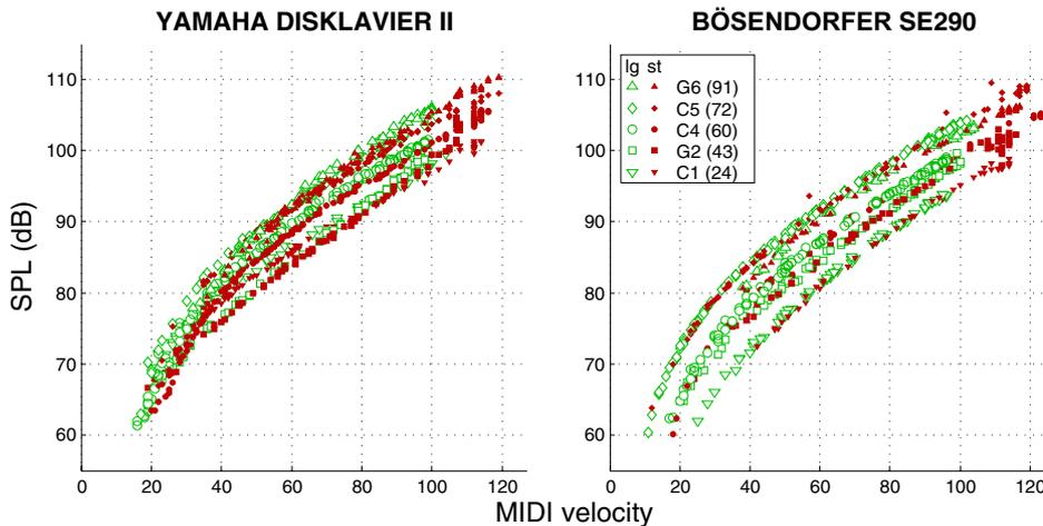
Figure 4: Peak sound pressure level (dB) against MIDI velocity as recorded by the two computer-controlled pianos. Different markers denote the five tones, different grey scales *legato* ('lg') and *staccato* ('st') touch.
