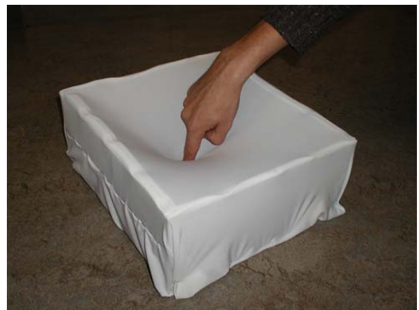
Figure 4: Haptic interface for the control of the Radio Baton. The interface is placed over the receiving antenna. Finger position in the 3-dimensional space is detected in real-time.
