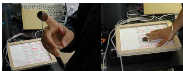
Figure 1: The thimble-based gestural controller for the Max Mathews' Radio Baton. It sends a radio signal from the fingertip to the receiving antenna.
