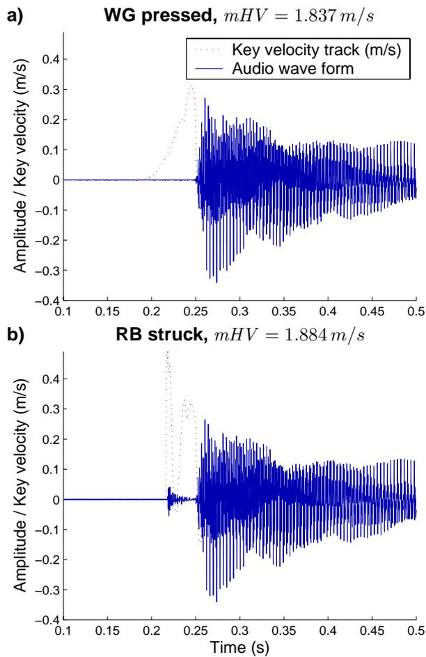
Figure 1: Audio wave form and key velocity pattern (dotted line) of two piano tones with similar hammer velocity. The upper tone was played with the finger initially resting on the key surface (a), the other struck from a certain distance above (b).
