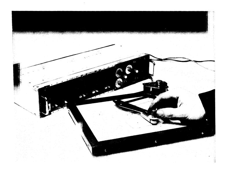
Fig. I-A-1. The new portable OVE Ib with electronics unit (including power supply, formant circuits, voice source, output amplifier) and function generator for control of F<sub>1</sub>, F<sub>2</sub>, F<sub>0</sub> and voice on/off.
