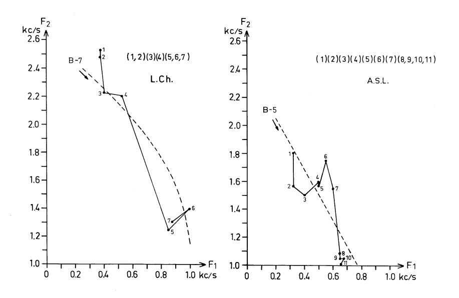
Fig. I-A-2. a. F<sub>1</sub> F<sub>2</sub> extent of stimulus trajectories (broken lines) and spectrographic measurements of F<sub>1</sub> and F<sub>2</sub> of the subject's mimicking response (solid points). The parentheses at the top of each diagram enclose mimicking responses judged to belong to the same category (phonetic identity being the criteria). Noise source excitation.
