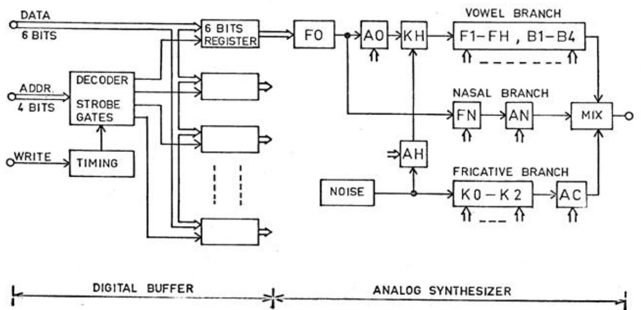
Fig. IV-A-2. Block diagram of the synthesizer with its digital control signal buffer.
