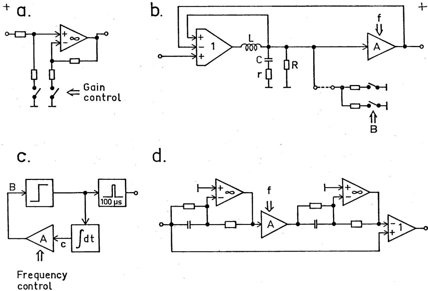
Fig. IV-A-3. a. One stage of a gain control module. Each module contains three cascaded stages.
