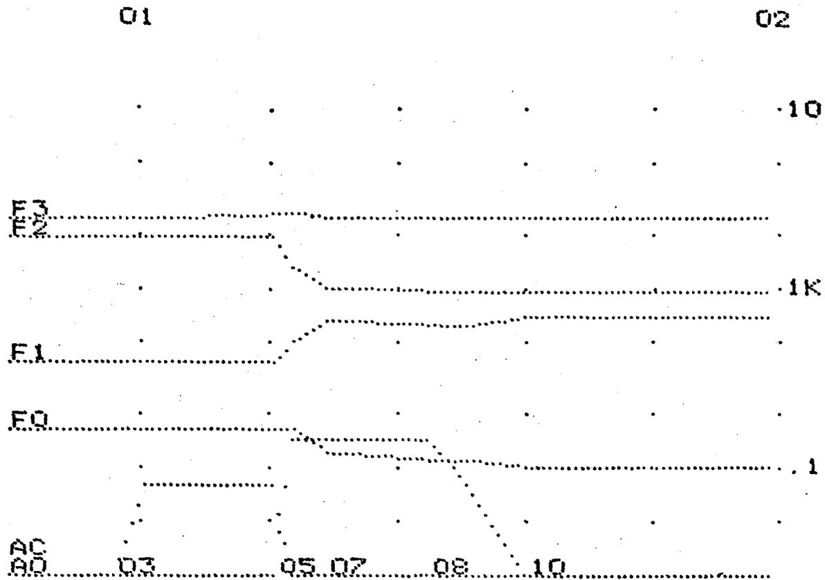
Fig. IV-A-4. Computer plot of some control parameters for the synthesis of /sa:/. Characters indicate: left, parameter names; top, time (seconds); right, frequency (kHz); and bottom, sample number.
