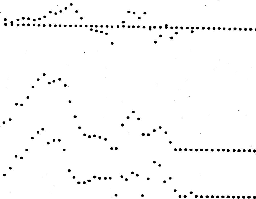
Fig. IV-A-5. Computer plot of spectra for the /a:/ of Fig. IV-A-4. From bottom to top: original sound, synthetic sound, and spectrum difference.
