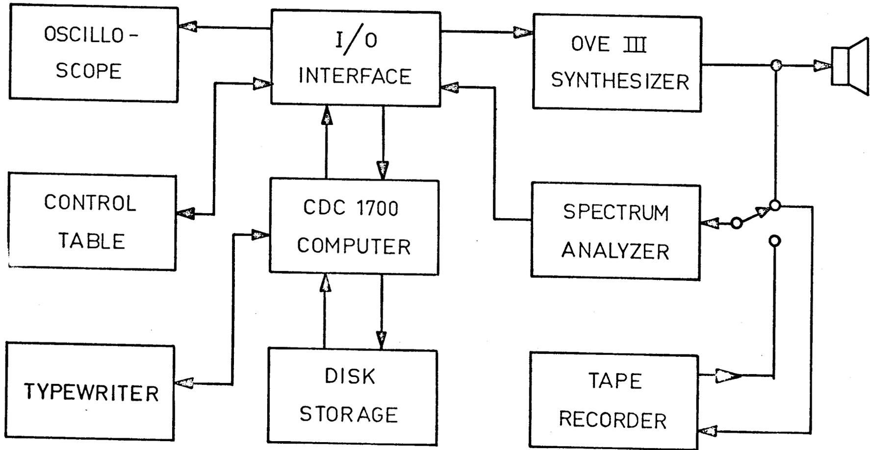
Fig. IV-A-1. Block diagram of complete synthesis setup.
