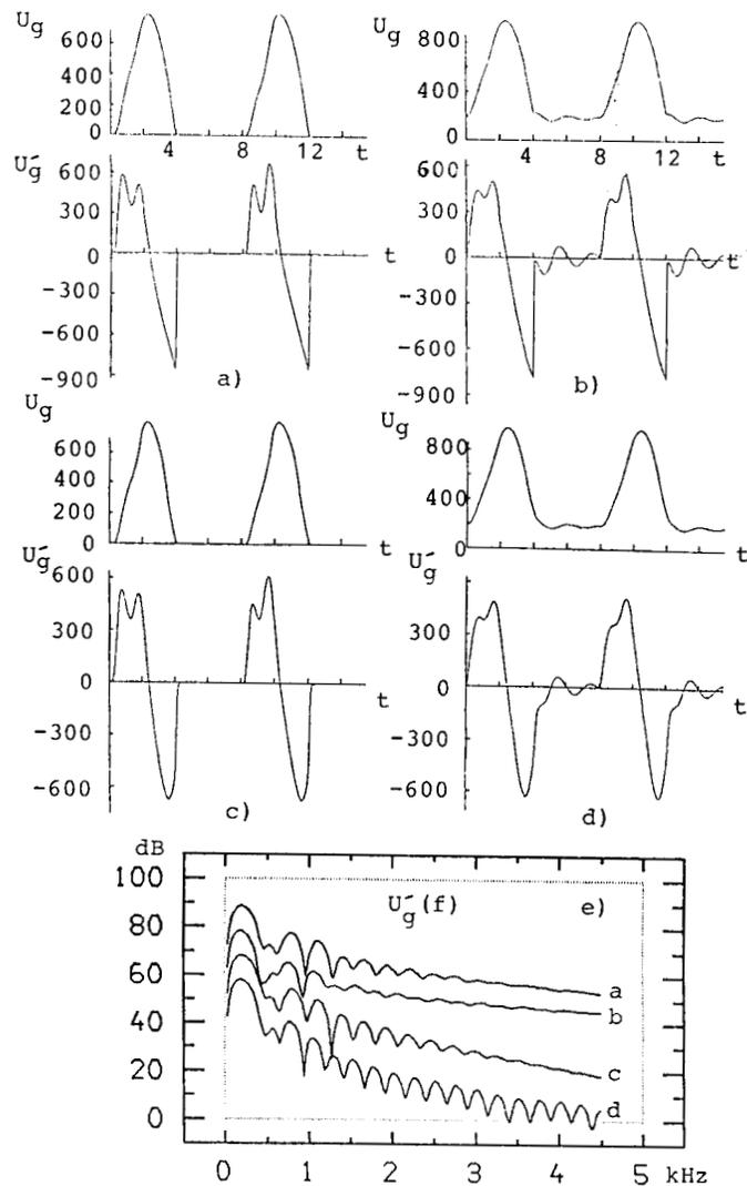
Fig. 7A. Leakage simulation. The acoustic load is modelled by as single formant.  $F/B=500/50$ ,  $L=5$  mH.
