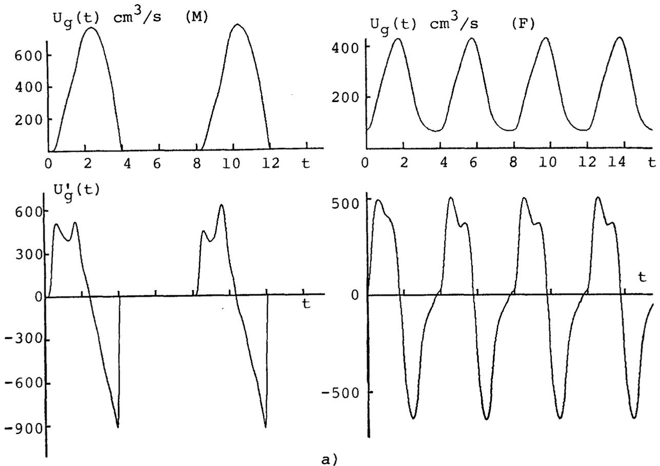
Fig. 10. An attempt to simulate male and female phonation of a neutral vowel. Male:  $A_g$  is modelled by a raised cosine function,  $T_o=8$  ms, open quotient is 50%,  $T_p/T_e=50\%$ .  $A_{gmax}=0.2$  cm<sup>2</sup>. Female:  $A_g$  is simulated by an LF-model,  $T_e=2.8$  ms,  $T_p=1.5$  ms,  $T_a=0.2$  ms,  $T_o=4$ ms.  $A_{gmax}=0.1$  cm<sup>2</sup>. This could represent a somewhat breathy phonation.
