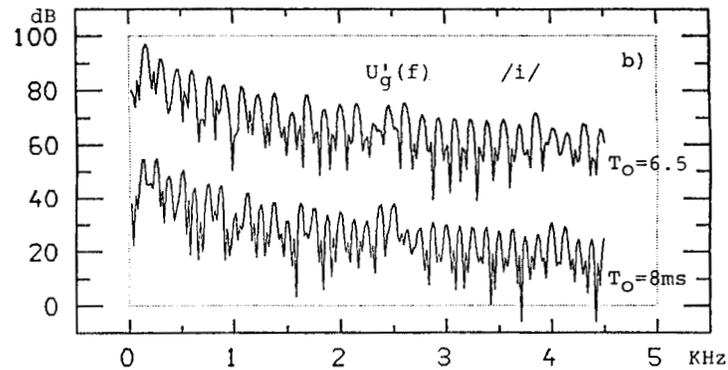
Fig. 5. a) The vowel /i/. Nonlinear superposition as a function of a varying duration of the closed phase. It should be noted that through  $T_O=7$  ms, the notch changes its location relative to the extra peak in the vicinity of 2.2 kHz.
