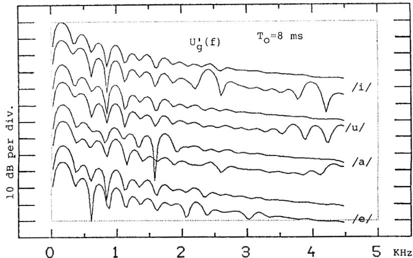
Fig. 6. The first and second pulse source spectra of different vowels: /i/, /u/, /a/, and /e/. The curve shift between the vowels is 15 dB. The first and second pulses are separated 10 dB. A small inherent difference in excitation level exists. It increases within the series /e/, /u/, /i/ and finally to /a/ with a total span of 1.5 dB. It is observed that the source spectra are inter-periodically different for each vowel.
