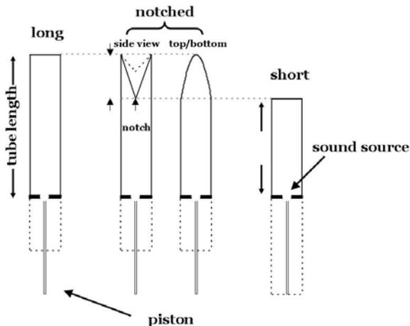
Figure 2. Cylindrical tubes used to study "spread lip" configurations.
