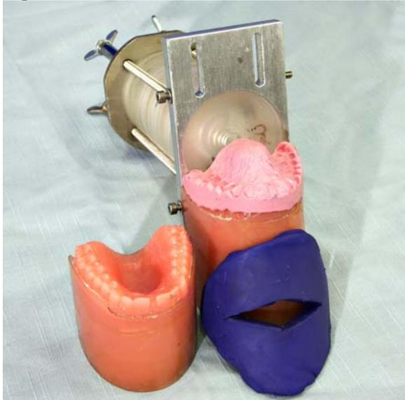
Figure 6. Components of the HACMOD replica of the vocal tract.: models of upper and lower teeth/jaws, lips, tongue shape and the posterior plexiglass unit.
