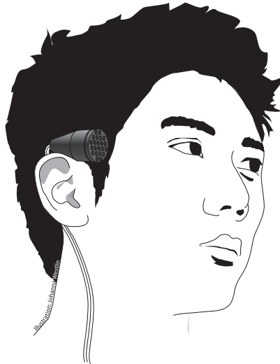
Figure 12: The microphone placement simulating the position of a BTE hearing aid, illustration J. Westlin
