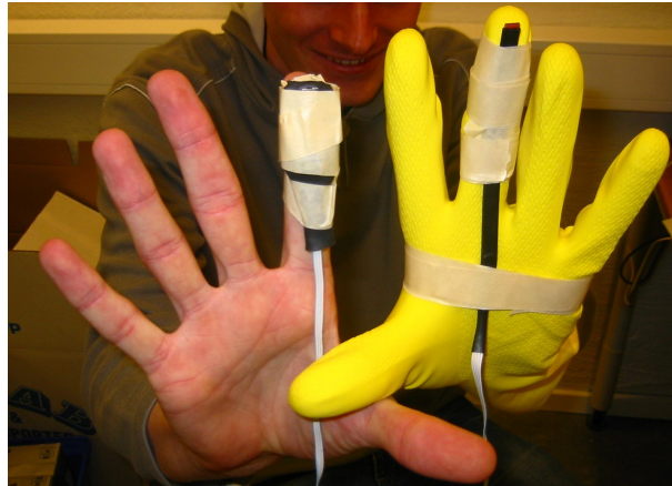
Figure 4: The second configuration showing the flexion sensor on the left hand and the magnetic field sensor on the right one.
