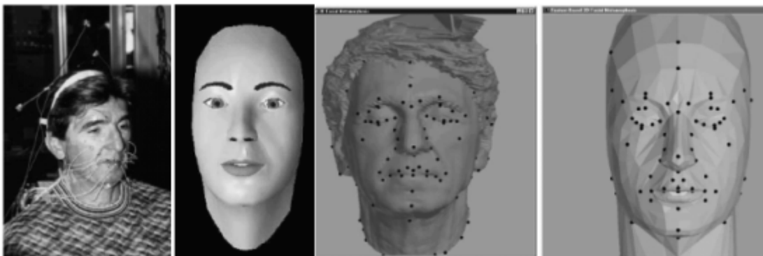
Figure 7: In the leftmost figure a training situation is shown; LED markers are used for measuring movements. The figures to the right show the alignment points placed on a laser scanned image and on the Baldi face.
