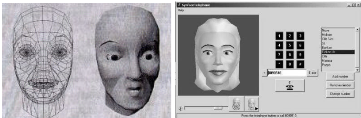
Figure 3: The visual interfaces of the Teleface project (left) and the Synface project (right) bear some resemblance to each other. To the left modelling by the Parke model is shown clearer. In the Synface project it is possible to choose from some different faces and the rest of the phone interface is built-in.
