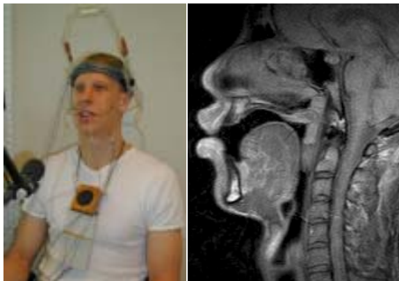
Different measurements for the 3D articulatory model (EPG, EMMA and MRI)
