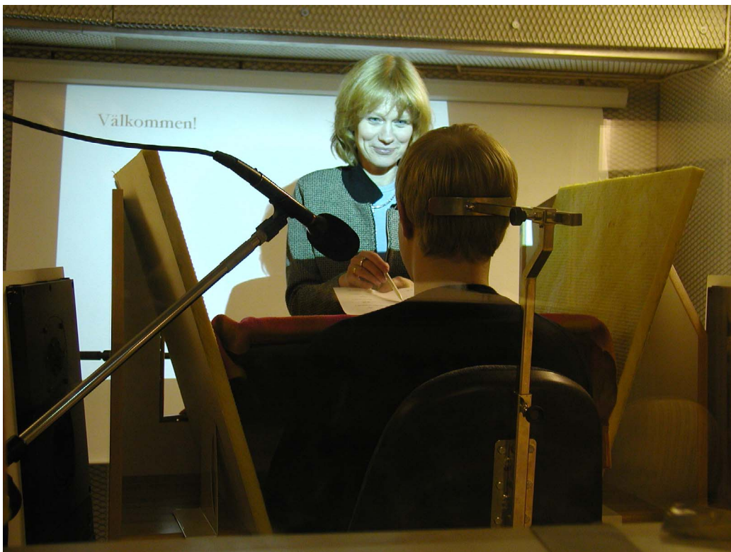
Experimental view from the voice load project, studying how normal speakers and voice patients use their voices in noisy workplace environments. A subject is being interviewed by voice therapist Maria Södersten about experienced voice strain, after having spoken loudly over recorded environmental noise. Note loudspeakers to the sides and the projection screen with instructions at the rear of the sound-proofed booth.
