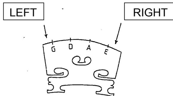
**Figure 8.15.** Measurement positions for vibration sensitivity, left and right.
