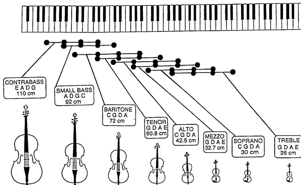
**Figure 8.11.** The new violin octet constructed Saunders, Schelleng and Carleen Hutchins and built by Hutchins - string tunings and relative sizes for the big bass, the small bass, the new cello (baritone), the tenor violin, the vertical viola (Alto), the mezzo violin, the soprano violin and the treble violin (after Hutchins).
