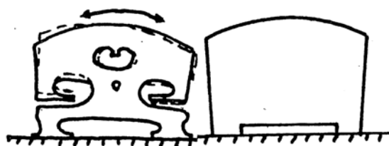
Figure 1: Normal violin bridge with first in-plane resonance at 3 kHz (left) and plate bridge with first in-plane resonance at 7.6 kHz (right).
