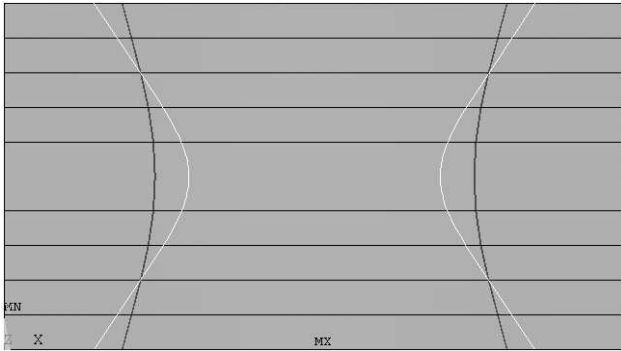
Figure 2: Reference material . Nodal lines for mode 2 (white curved lines represent measured nodal lines and black calculated).
