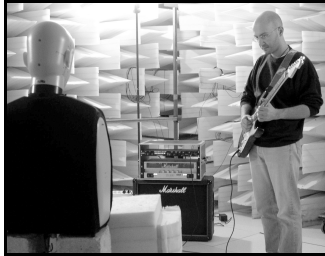
Figure 2: HATS and guitarist in the anechoic chamber.
