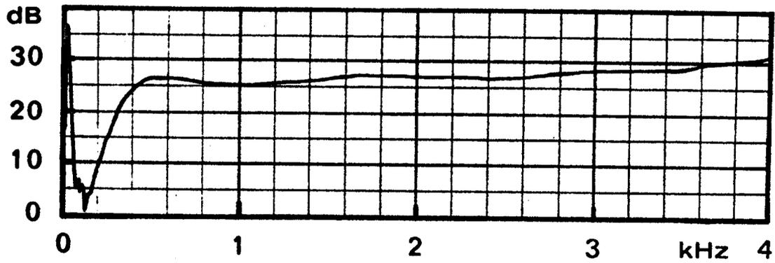
Fig. I-B-2. Response curve for the sound source with an 11 cm probe-tube connected.
