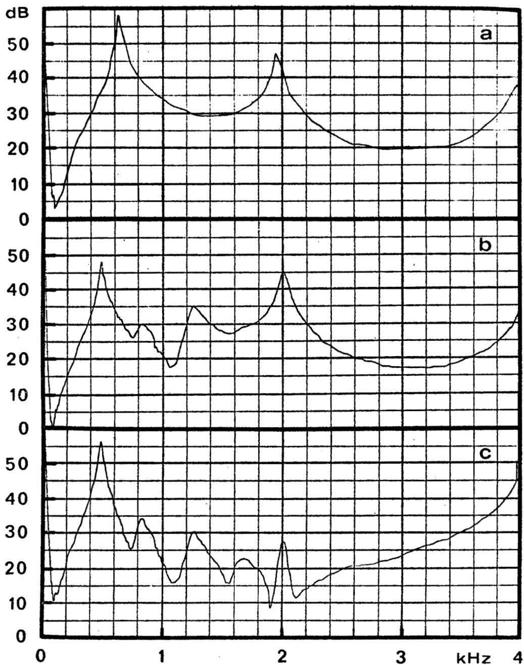
Fig. I-B-5. Response curves for a twin tube model of the nasal tract, a; without shunting cavities, b; with two shunting cavities corresponding to the maxillary and frontal sinuses. In c the source is asymmetrically placed simulating asymmetry in the two nasal passages.
