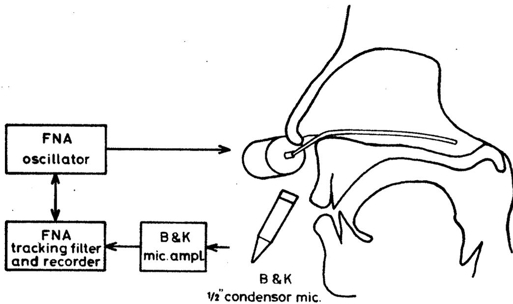
Fig. I-B-3. The experimental setup for recording of the transfer function of the nasal tract.
