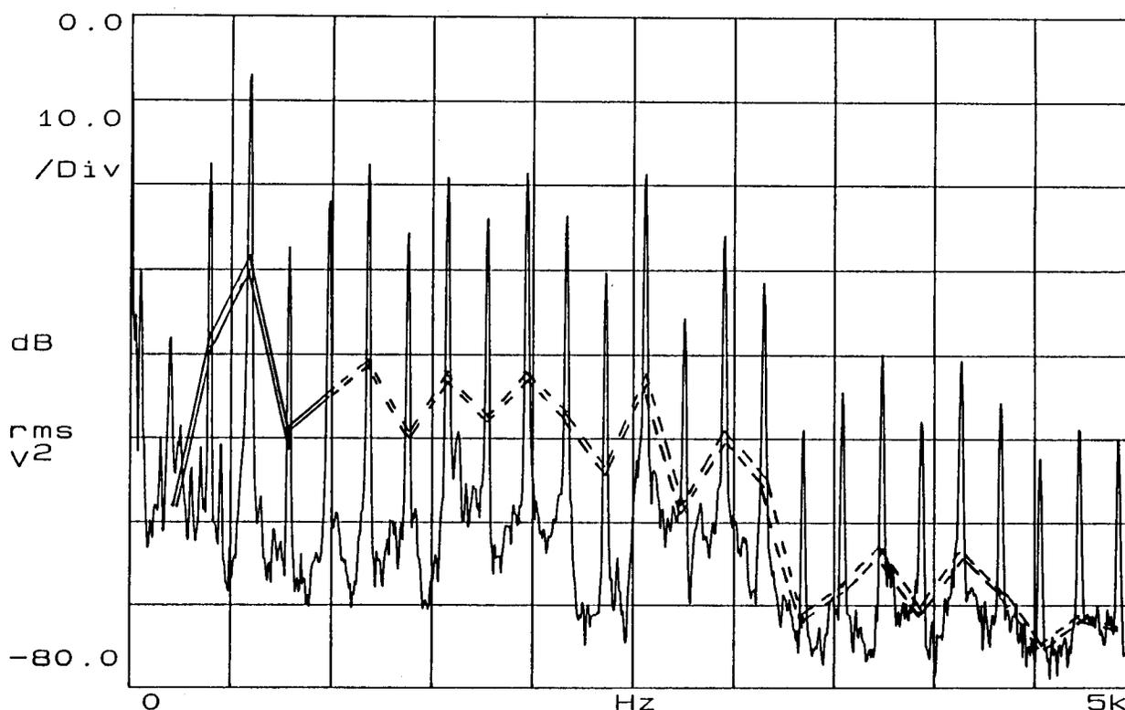
Fig. 2. *Spectrum of a played open G-string (196 Hz) measured at the left ear of the player with maximum allowed noise levels not to mask partials (assuming an analysis bandwidth of 1 Hz). Full lines mark the region where the critical band noise level is adaptable and broken lines where the partial separation noise level is adaptable.*
