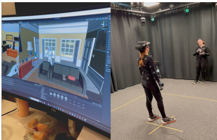
Figure 6.4: Overview of the VR recording setup. Left: the Unity-based AI2-THOR simulator, where the actor’s motion-capture data is streamed over a network connection. Right: the motion-capture studio with two actors engaged in conversation.
