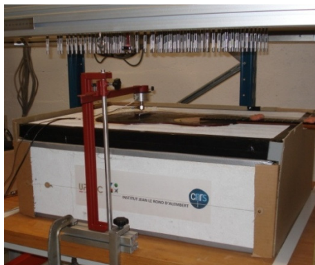
Figure 1. Experimental setup. The guitar is located in a baffling box, the impact hammer excites the soundboard on the bridge, the strings are muffled. The microphone array is located on a parallel plane to the soundboard.
