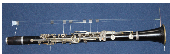
Figure 2. The measurement patches mounted on the nylon filaments. Measurement positions are indicated by arrows.
