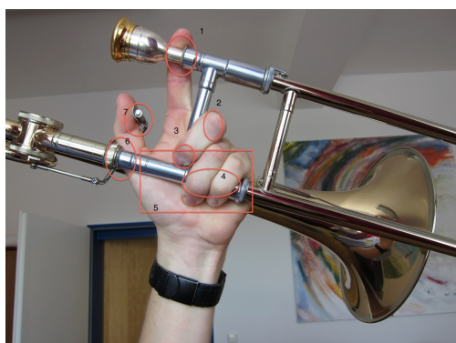
Figure 3. Contact points between the trombone and the fingers of the player. The right hand is missing in this picture but also measured. The numbers indicate each contact point at which sensors are attached to the instrument.
