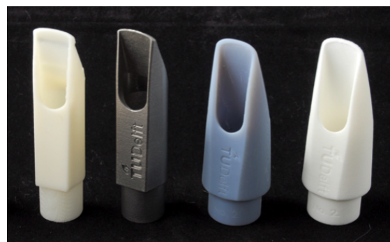
Figure 1: Preliminary mouthpiece models produced using different 3D printing technologies and materials.
