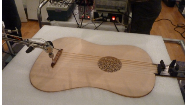
Figure 3. Experimental setup for top plate impulse response measurement. The instrument is installed in its baffle, the strings are muffled. The excitation hammer and the reference accelerometer are in place.
