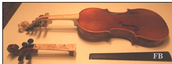
Figure 10: The Guarneri model violin fitted with a HF neck. The violin fingerboard (FB) was carved flatter and hollowed out for the sympathetic strings on the HF. Response curves were measured for each step in the working process.
