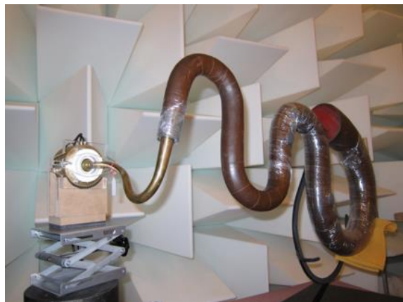
Figure 1. Experimental set up used to measure the input impedance of historical Serpents.
