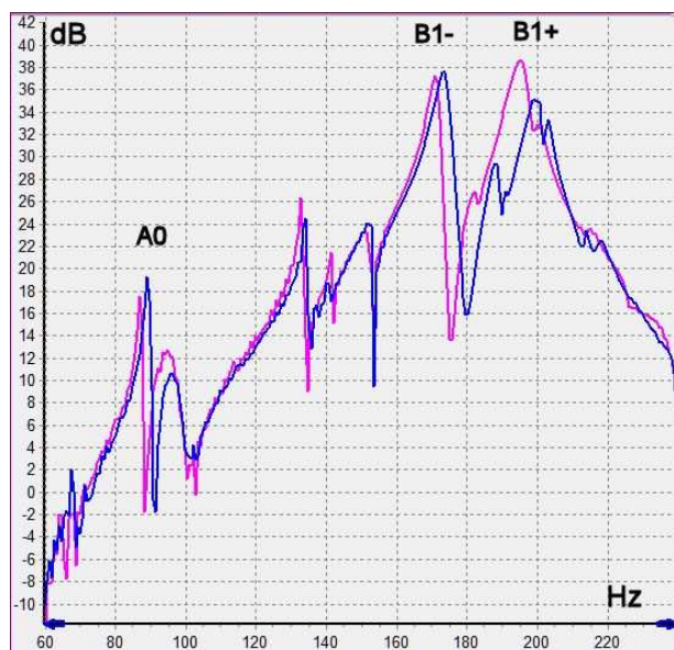
Figure 6. Cello Body Modes for standard Set-up 1 (pink) and Set-up 2 (blue) with long tailpiece T2 and shorter after length. Same tail cord length for both.
