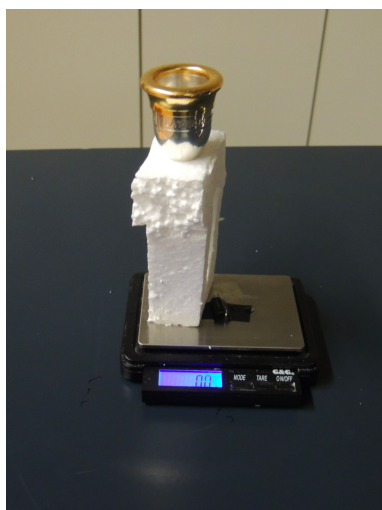
Figure 5. Setup with a scale for pressure sensor calibration.
