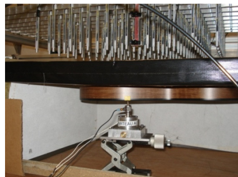
Figure 3. Experimental setup for holographic modal analysis.
