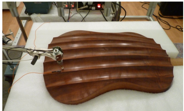
Figure 4. Experimental setup for the back impulse response measurement. The instrument is installed in its baffle. The excitation hammer and the reference accelerometer are in place.
