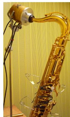
Figure 8. Photo of the saxophone input impedance measurements.
