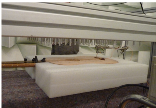
Figure 5. Experimental setup for the top plate impulse response measurement. The microphone array is located at a distance z_h = 103 mm from the soundboard.
