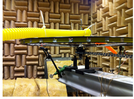
Figure 2. Fixation of the Hummer on the Wheel and detection of wheel rotation.
