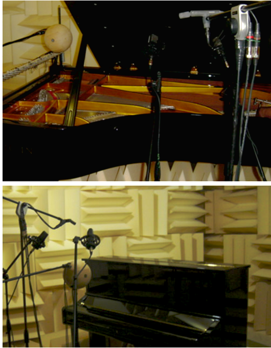
Figure 2. Microphone setup during the recording sessions of Seiler mod. D (top) and Yamaha YUS1 (bottom).
