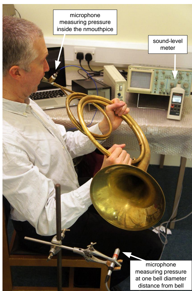
Figure 3. Experimental set up, showing the positions of the microphones and sound-level meter.
