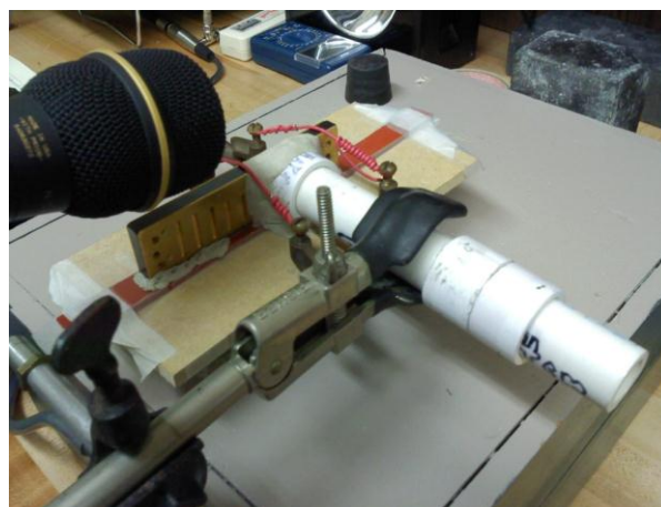
Figure 4. Harmonica mounted on wind chamber with attachment of variable length PVC pipes.
