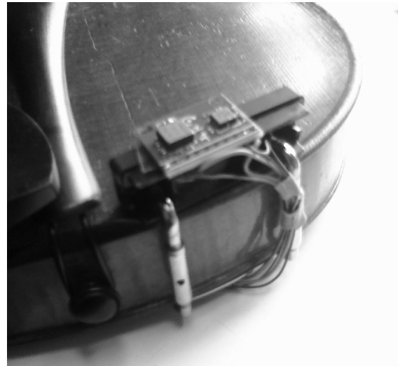
Figure 3. Shown is the sensor board attached to the violin. This typical "chin rest" mount allows stable fixation at the same position on every violin.
