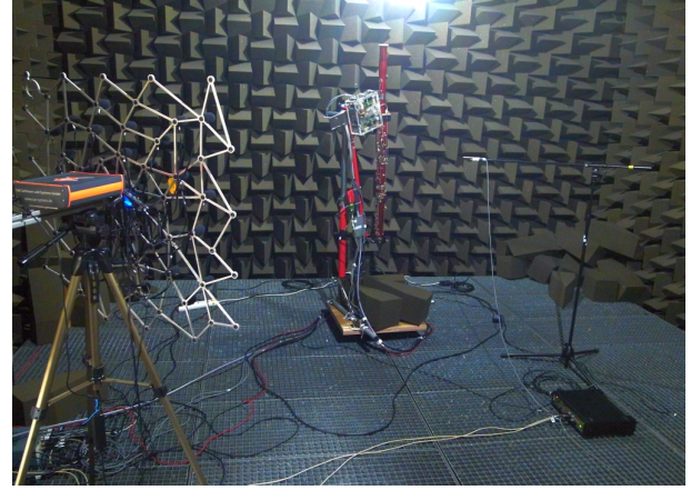
Figure 1: Bassoon with artificial mouth excitation mounted vertically on a turntable. Left and right of the bassoon are the acoustic camera and the close microphone (1.2 m). The far microphone is not shown.
