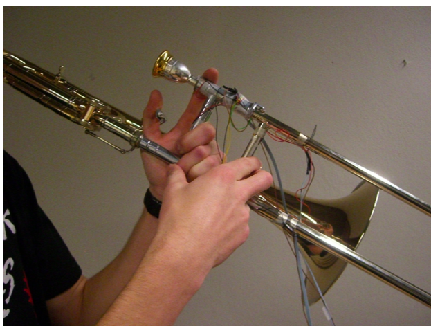
Figure 1. Trombone with eight pressure sensors fixed to the instrument. The contact points (left hand, right hand, and lips) between the musician and the instrument are covered with flexible FSRs to measure the applied pressure.
