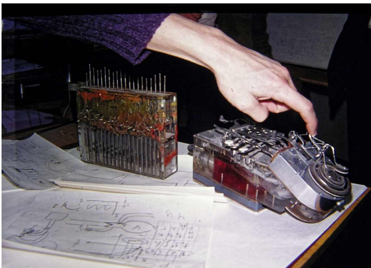
Details of the Novosibirsk synthesizer. The vocal tract model to the left.
